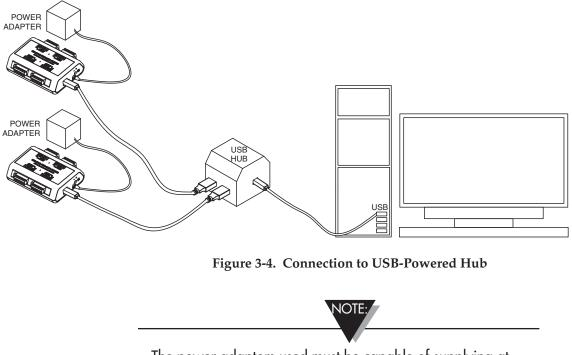
The power adaptors used must be capable of supplying at least 500 mA and have a voltage rating of +7.5 to +12 Vdc.
